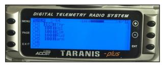
3.The default channel map for Larva X Frsky version is TAER1234, please make sure your transmitter is matched, otherwise it will can't be armed. Toggle the AUX1 Switch ,the Green LED on the flight controller will getting to be solid, this indicates the motor was armed. And also you can found "Armed" displayed on your FPV Goggles or the FPV Monitor. Please make sure keep the Larva X level before arming. Be careful and enjoy your flight now!
