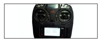
3. The default channel map for Larva X DSM2/X version is TAER1234, please make sure your transmitter is matched, otherwise it will can't be armed. Toggle the AUX1 Switch ,the Green LED on the flight controller will getting to be solid, this indicates the motor was armed . And also you can found "Armed" displayed on your FPV Goggles or the FPV Monitor. Please make sure  $keep\ the\ Larva\ X\ level\ before\ arming\ . Be\ careful\ and\ enjoy\ your\ flight\ now\ !$
