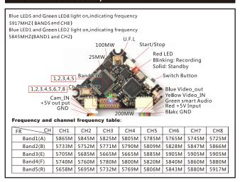
The DVR will recording automatically when power on.
