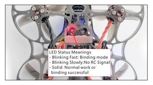
2.Turn on your transmitter and Choose AFHDS-2A for the receiver mode(Some Flysky transmitter default setting is AFHDS-2A). Then ENTER RX bind, if bind successful the Red Led at the bottom of the flight controller will getting to be solid. Then reconnect the USB and exist bind mode. Now move to receiver tab of the Betaflight configurator to check the receiver works
