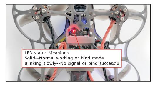
2.Turn on your transmitter and then move to Model setup ,select D8 mode and then ENT "bind" to binding with the onboard receiver , if bind successful the Red Led at the bottom of the flight controller will starting to blinking slowly . Then reconnect the USB and exist bind mode . Now move to receiver tab of the Betaflight configurator to check the receiver works
