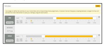
2. Set Arm/Disarm switch for your Flysky Radio: Move to the Aux.channels interface, Set "SWA" or "SWB" or "SWC" switch etc. for Ch5 to ARM/DISARM the motor.
