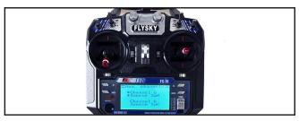
3.The default channel map for Mobula6 Flysky version is AETR1234, please make sure your transmitter is matched, otherwise it will can't be armed. Toggle the AUX1 Switch, the Green LED on the flight controller will getting to be solid, this indicates the Mobula6 was armed. And also you can found "Armed" displayed on your FPV Goggles or the FPV Monitor. Please make sure keep the Mobula6 level before arming .Be careful and enjoy your flight now!
