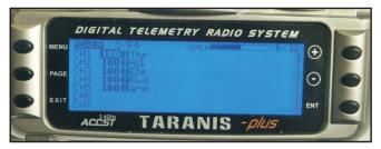
3.The default channel map for Mobula6 HD Frsky version is TAER1234, please make sure your transmitter is matched, otherwise it will can't be armed. Toggle the AUX1 Switch ,the Green LED on the flight controller will getting to be solid, this indicates the motor was armed . And also you can found "Armed" displayed on your FPV Goggles or the FPV Monitor. Please make sure keep the Mobula6 HD level before arming .Be careful and enjoy your flight now!
