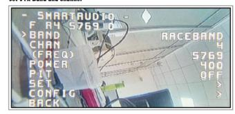
3).Enter into ExpressLRS.lua then choose VTX administrator menu; Change Band, channel value, power level that you needed and then final Send vtx . Some times need to cycle power for the drone to make it effective.
