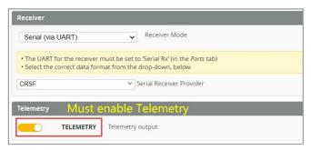
2) Please make sure your ExpressLRS tx module firmware is v3.x.x. And go to ExpressLRS.lua from "TOOLS" menu of your radio transmitter. Then hit [Bind] to binding with the onboard ExpressLRS receiver. The RGB LED should blinking slowly first then turn to solid, that means binding was successfully.
