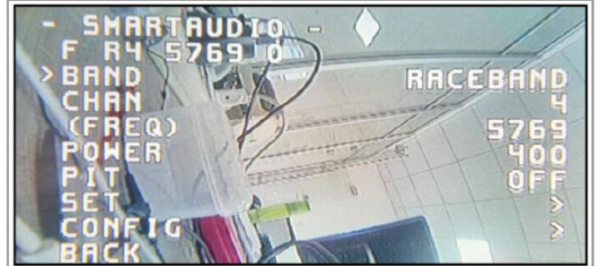
3).Enter into ExpressLRS.lua then choose VTX administrator menu; Change Band, channel value, power level that you needed and then final Send vtx . Some times need to cycle power for the drone to make it effective.
